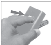
Push to release batteries
